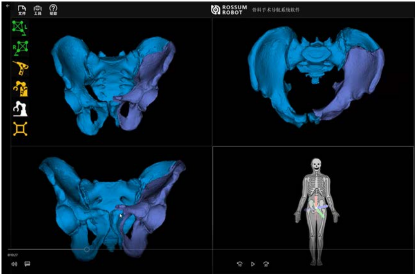
Fig. 4. After image registration, the position of the pelvic can be tracked in real-time and displayed on the screen.
